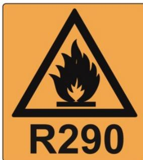
This appliance contains the **flammable refrigerant R290**. Any maintenance operation on the refrigeration circuit must be performed uniquely by specialized personnel which must have adequate skills and the certification required by the F-GAS directive.
