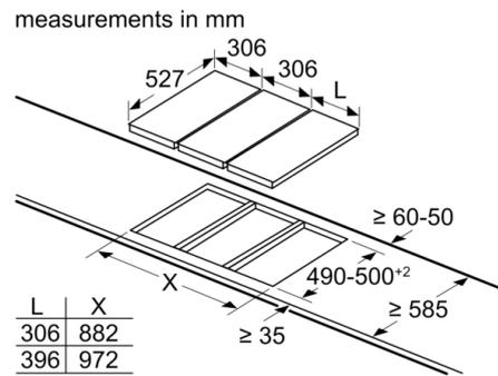
When installing two or more Domino units side-by-side, one or more assembly kits are required (2 units = 1 assembly kit, 3 units = 2 assembly kits, etc.).
