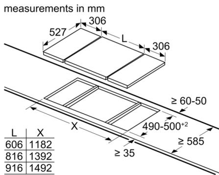
When installing two Domino units right next to a hob, two assembly kits (HEZ394301) are required.
