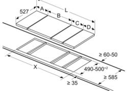
If two or more elements are installed right next to one another, one or several installation kits are required (2 elements 1 installation kit, 3 elements 2 installation kits, etc.).
